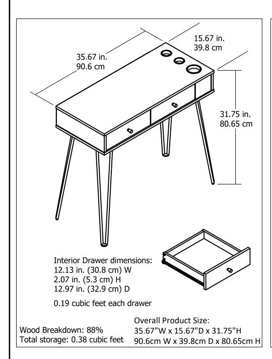
70 lbs 31.8 kg 20 lbs 9.1 kg (each drawer) **Maximum Weight Capacities** Unit Weight: 35 lbs. (15.9 kg)
